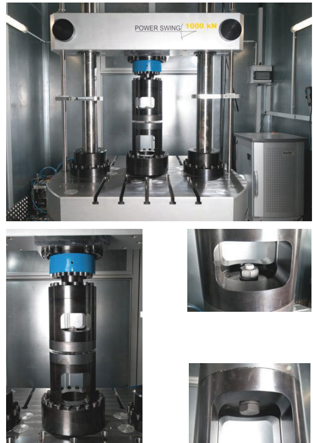
Fig. 7. Test set-up for high-strength bolt-sets M36 under pure axial loading in a high frequency pulsator
