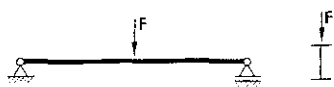
Fig. 1. The test specimen for the transient-state tests: a beam simply supported with a single load in the midspan.
