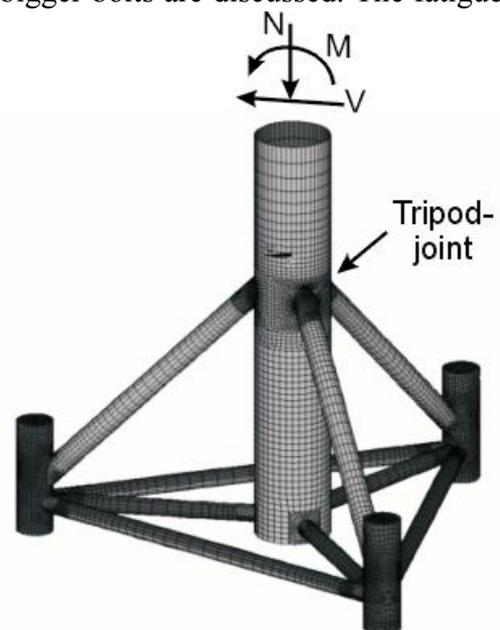
Fig. 11: FE-model of a tripod
