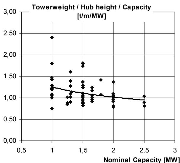
Fig. 4 Referred weights of steel tube towers of 68 wind turbines in the MW-class; source: Windkraftanlagenmarkt 2002 [5]
