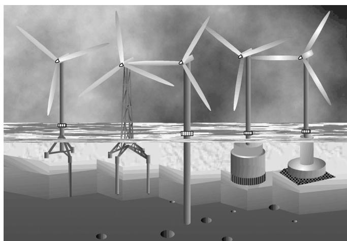
Fig. 5: Concepts for support structures for offshore wind turbines © GIGAWIND
