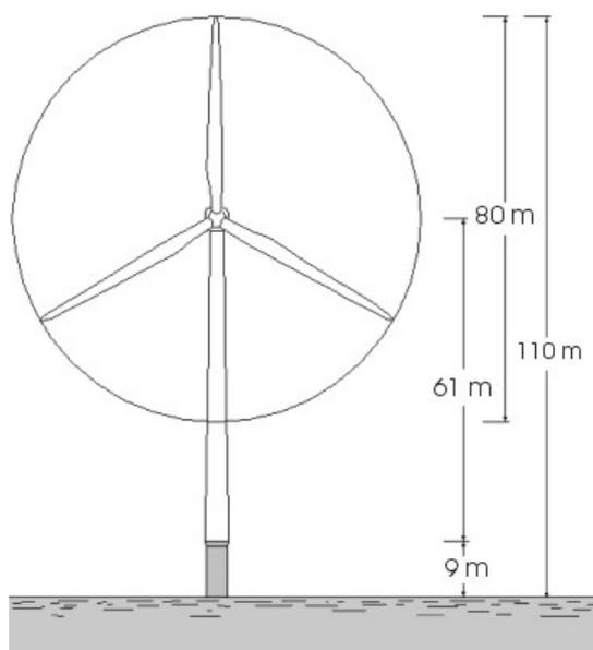
*Fig. 6 Dimensions of the wind turbines in Danish Horns Rev
