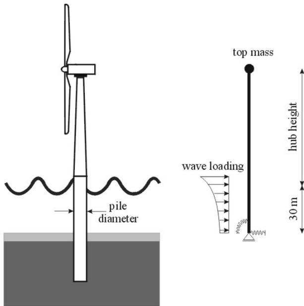
Fig. 8: Numerical model for calculations
