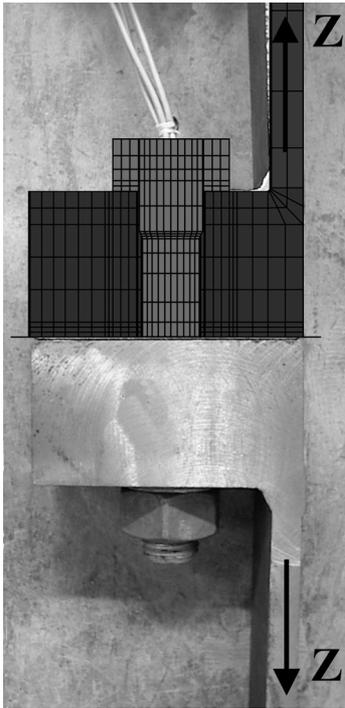
Fig. 10: FE-Model and flange segment
