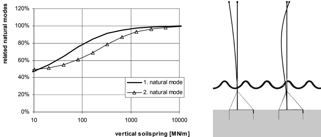
Fig. 7: Influence of the vertical soil spring to the first two natural modes of a tripod foundation [10], illustration of the affiliated vibration modes
