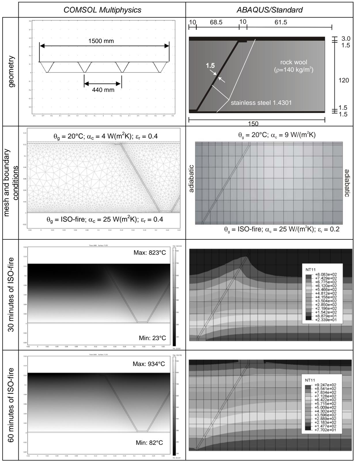
Fig. 5 – Thermal modelling in COMSOL and ABAQUS.
