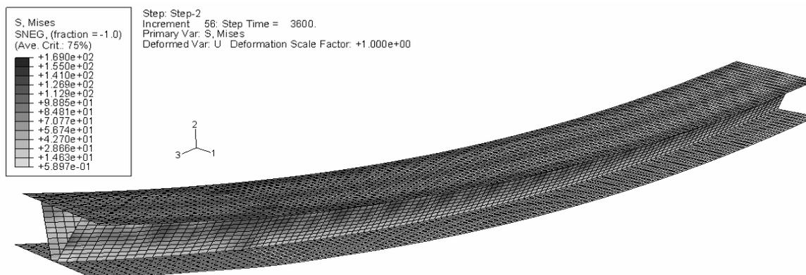
Fig. 10 – Deformed *ABAQUS*-model and Mises-stresses after 60 minutes of ISO-fire (no amplification).
