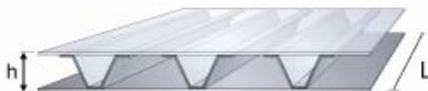
Fig. 1 – Stainless steel sandwich panel.
