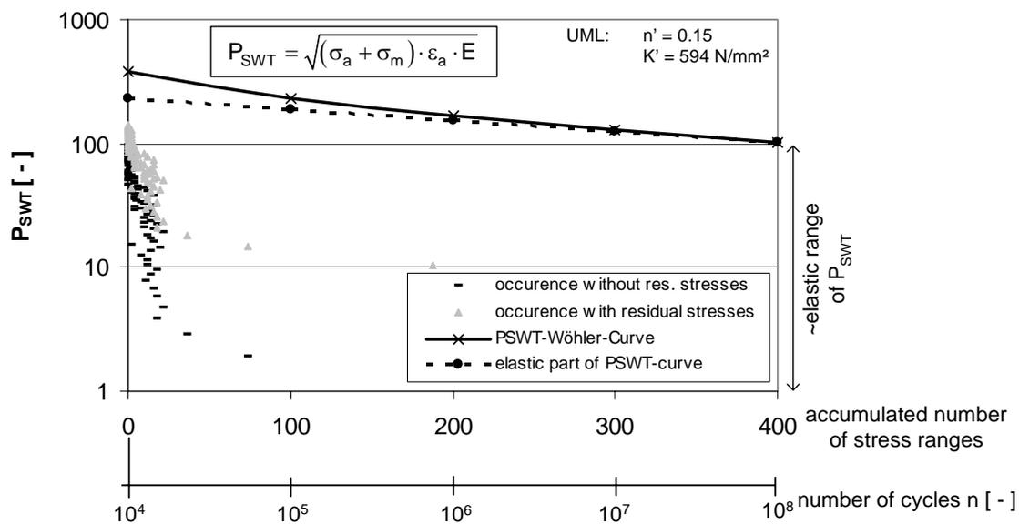
Figure 8:  $P_{SWT}$  damage parameter for the stress ranges of an exemplary time-history near the cut-out wind speed for the detail in Figure 6
