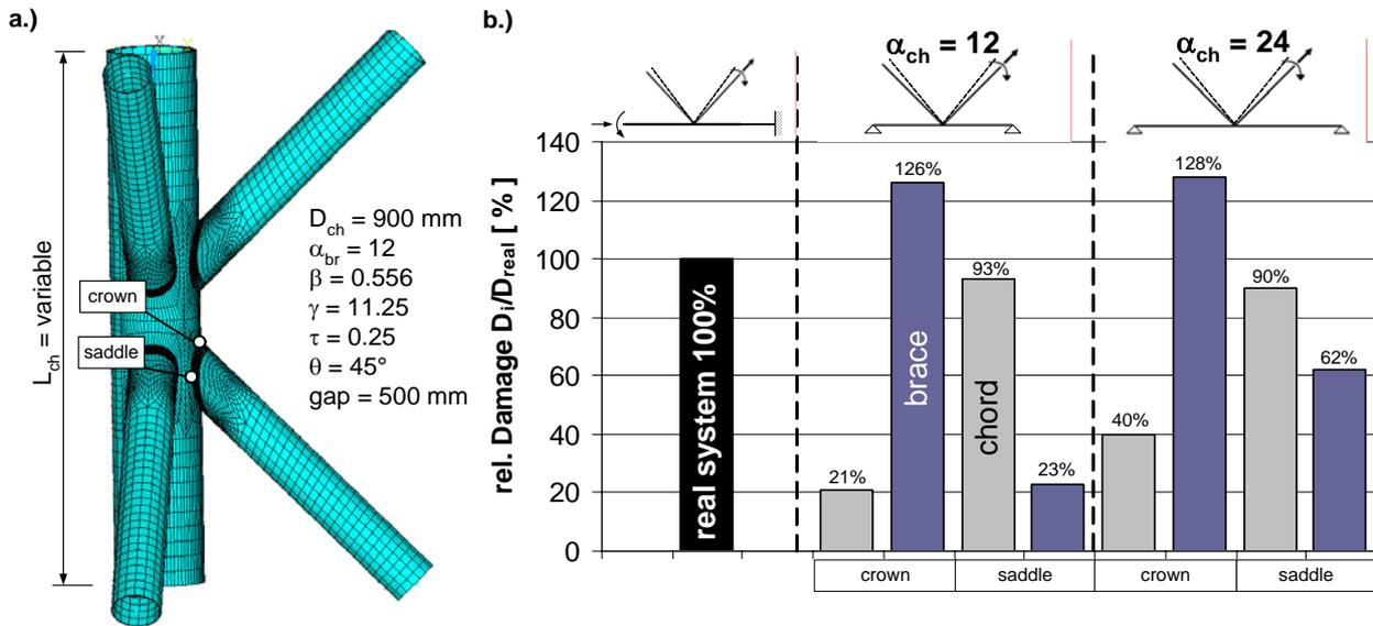
Figure 6: a.) Model of 90°-DK-joint; b.) Related damage at real and simplified system
