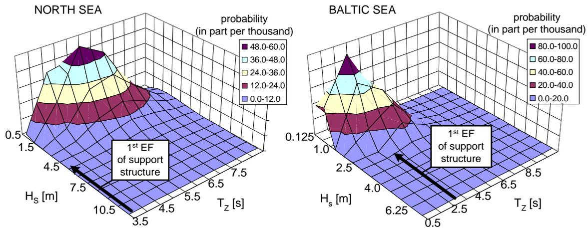
Figure 5: Wave scatter diagrams for two different German locations
