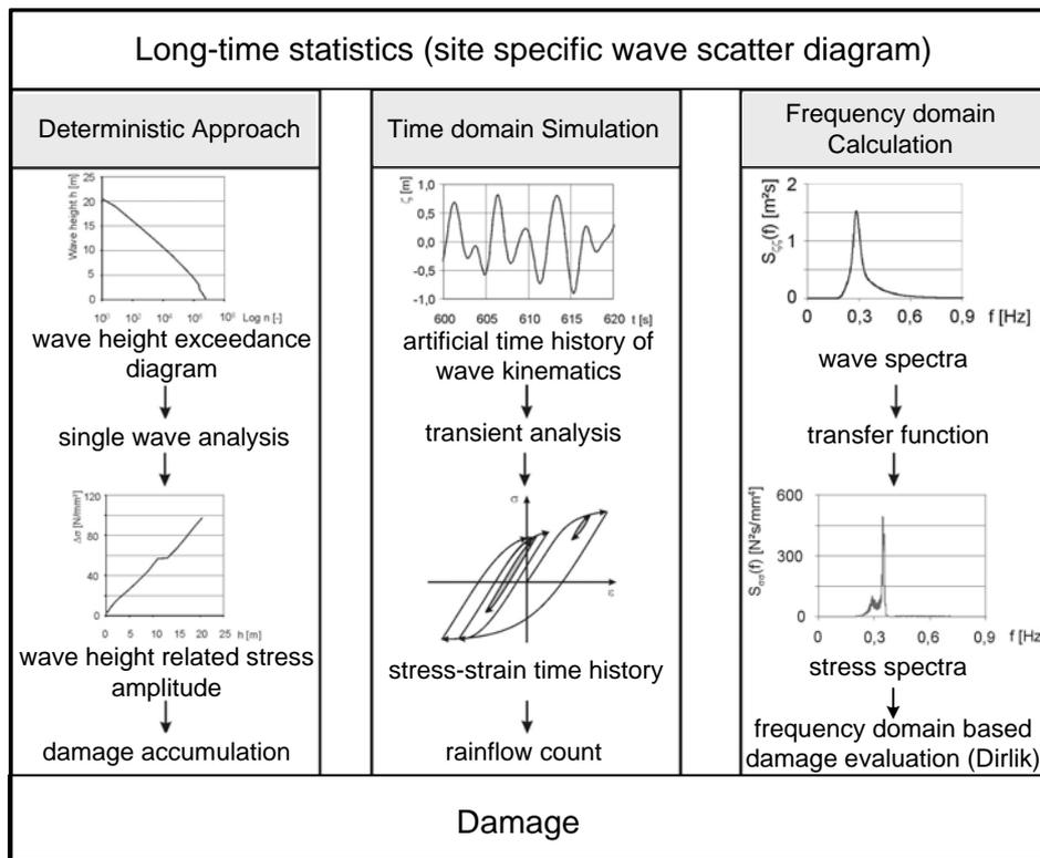
Figure 4: Fatigue design approaches acc. to Kleineidam (2004)
