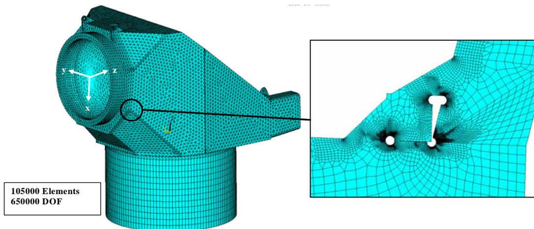
Figure 7: Analysed part of the welded machine carrier
