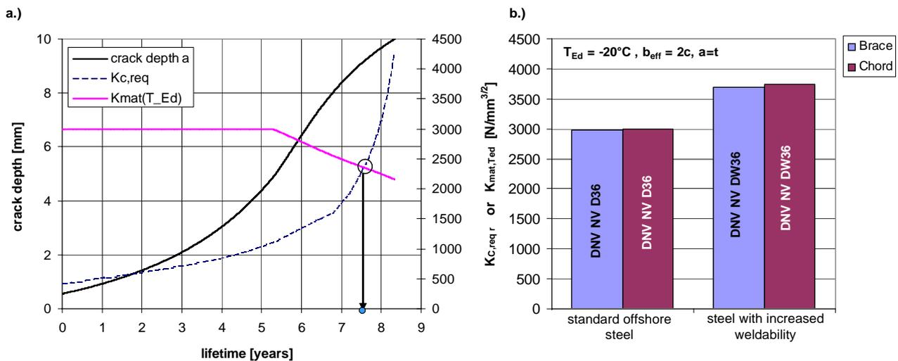
Figure 9: a.) crack depth/required fracture toughness vs. lifetime for the brace saddle location of the DK-joint Figure 6; b.) required fracture toughness of two different steel materials acc. to DNV (2004) for a joint in the splash zone ( $T_{Ed} = -20^\circ\text{C}$ )
