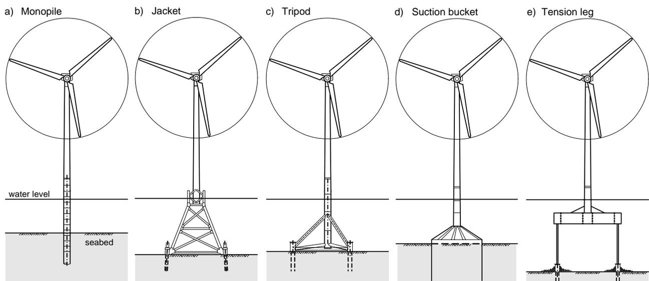
Figure 1: Concepts for the support structures of offshore wind energy converters acc. to (Schaumann et. al 2004)
