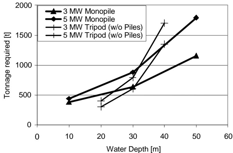
Figure 2: Water depth dependency of monopile and tripod weights for a 3 and 5 MW turbine (Schaumann & Böker 2005)
