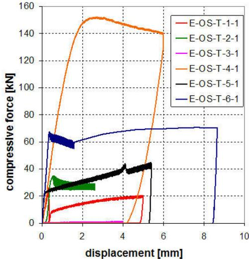
Fig. 6 Ultimate limit states for different core materials without shear keys
