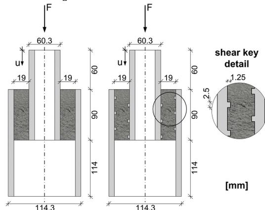
Fig. 4 Geometry of test specimens without (left) and with shear keys (right)
