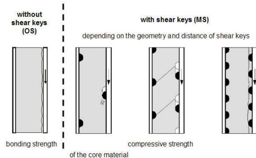
Fig. 9 Failure modes in single shear connections with and without shear keys
