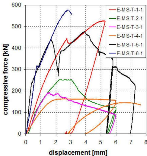
Fig. 7 Ultimate limit states for different core materials with shear keys
