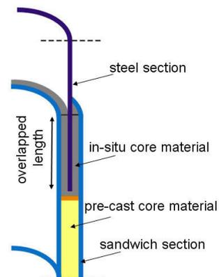
Fig. 2 A new connection for tower sections
