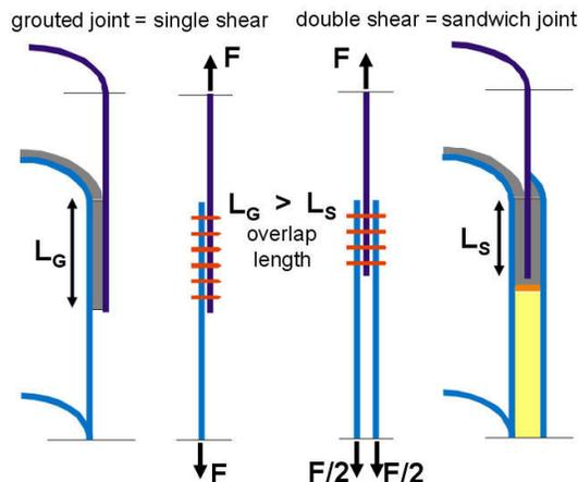
Fig. 3 Single and double shear connections
