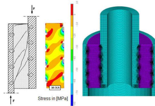
Fig. 8 Cracks in core materials and stress concentration in numerical models [5]
