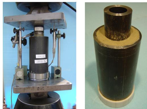
Fig. 5 Test setup and specimen
