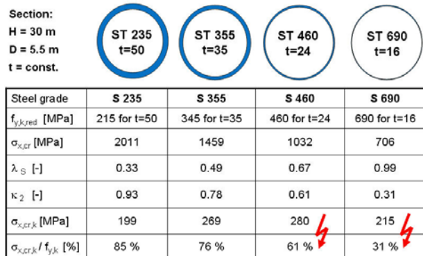
Figure 1: Comparison of tower sections with various steel grades with regard to shell buckling
